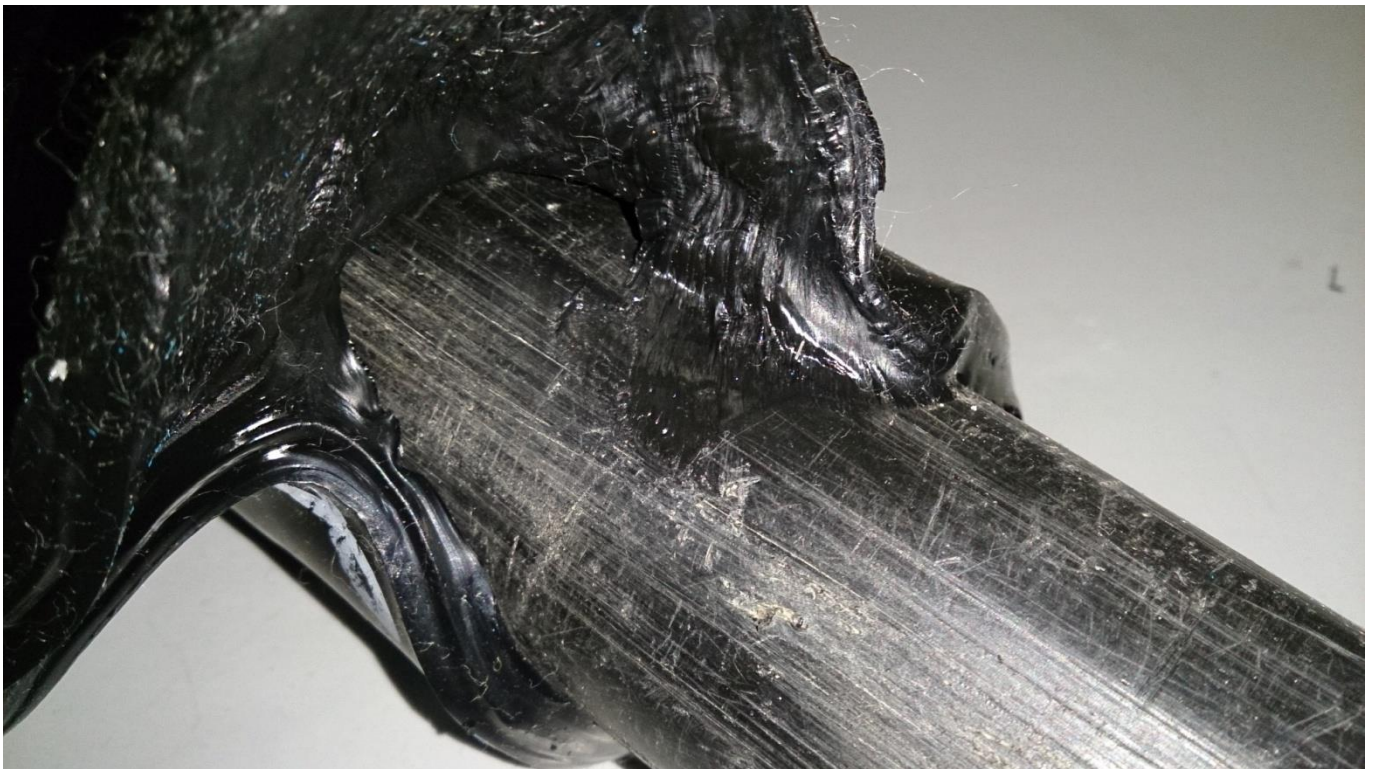
Fig.7. Adhesion of HDPE pipe to the surface of the cable outer sheath.
