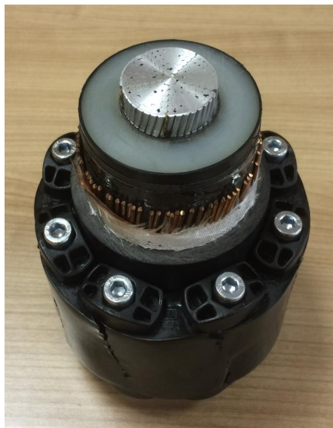
Fig.2. Single-core cable with a ring seal on it.
