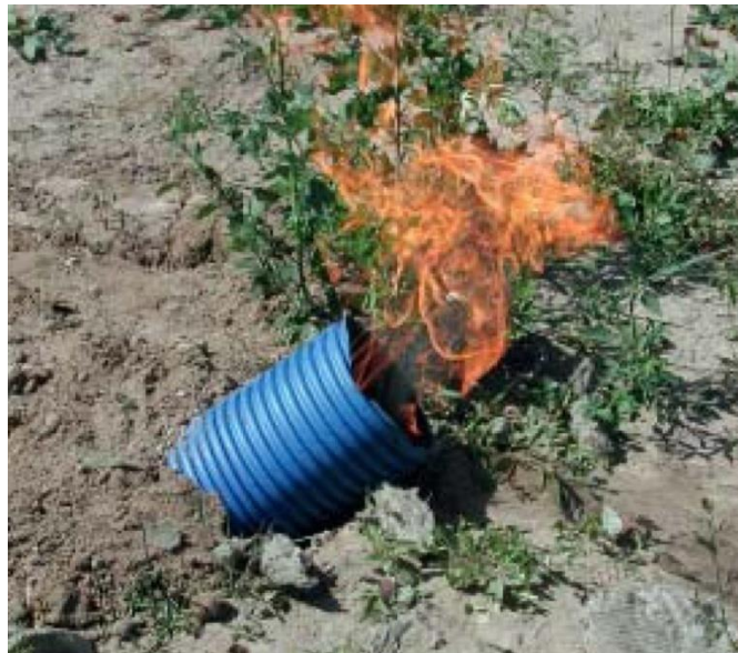
Fig.5. Blue-painted corrugated pipe made of ordinary polyethylene. It does not have an internal nonflammable (NF) layer and seals. The solution is designed for CL up to 1 kV.
