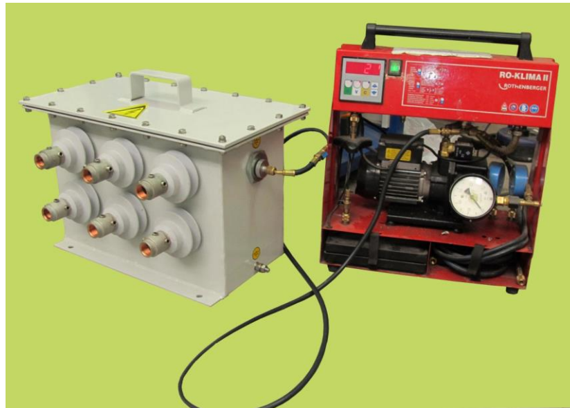
Fig.3. Factory tests of the link box for tightness.
