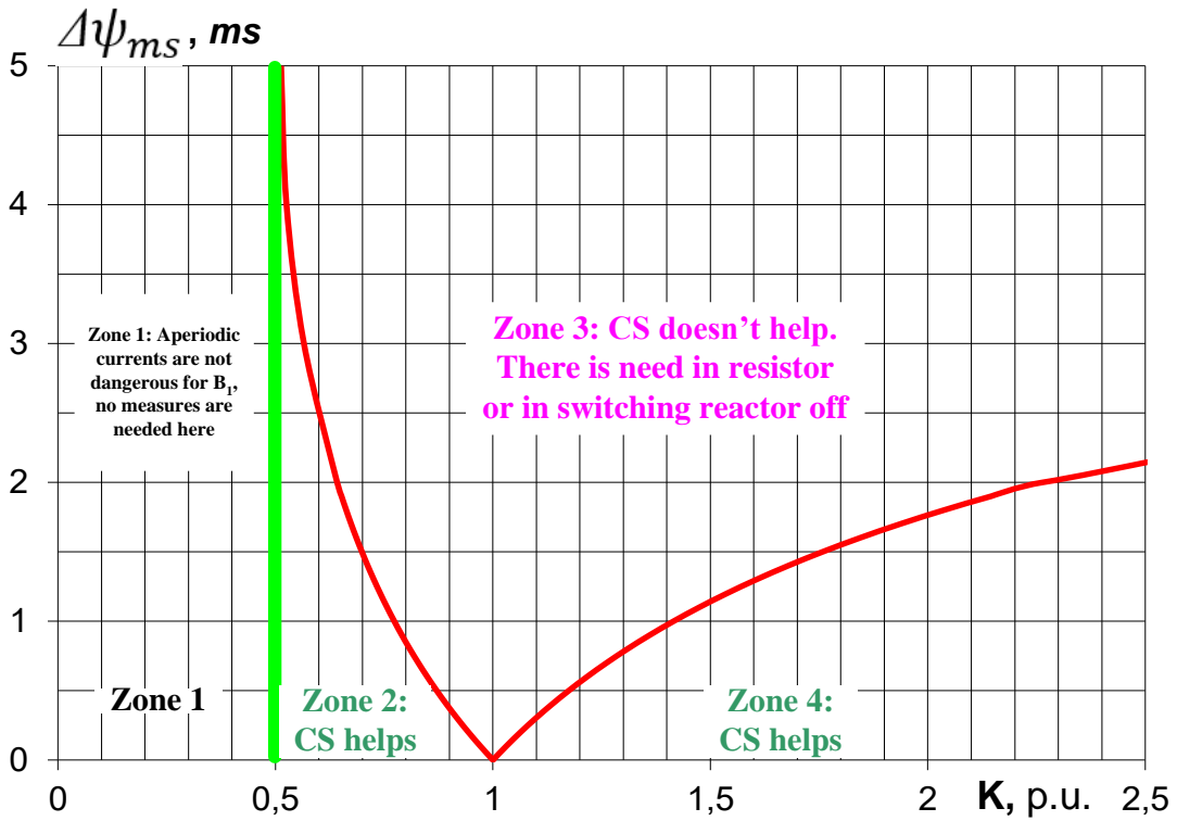
Fig.3. Requirements to the accuracy \Delta\psi of controlled switching depending on the compensation coefficient K of the charging power of typical 500-750 kV overhead lines.
